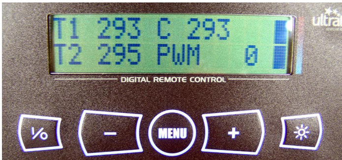
If set the Fog output stops when fluid gets low (F indicator on main screen).
