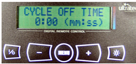
Menu screens for timer on/off function with remote control only. DMX control ignores these setting.
