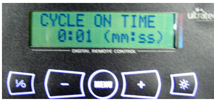
Menu screens for timer on/off function with remote control only. DMX control ignores these setting.
