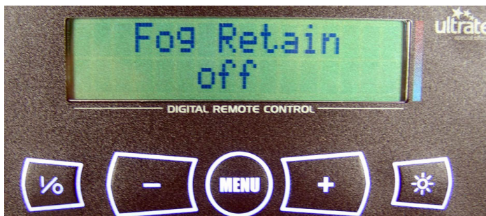
If set the Fog output stops when fluid gets low (F indicator on main screen).
