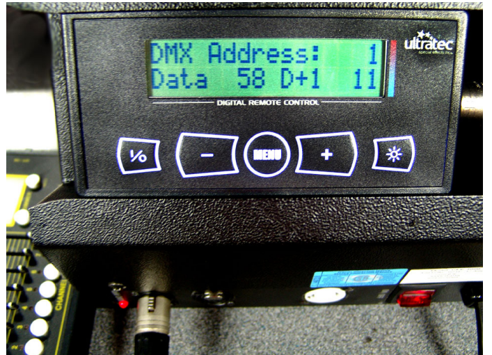
DMX address selection screen. This shows DMX set to channel 1. Channel 1 data is 58 (0-255) channel 2 is 11.
